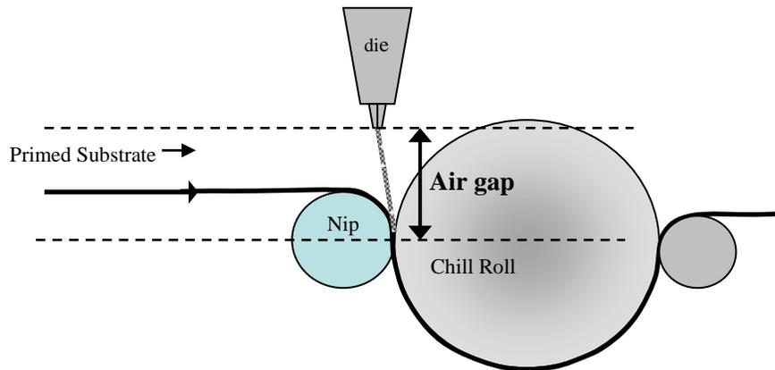
Field experience has shown us that for LDPE, the best time in the air gap (TIAG) is in the range of 60 to 120 milliseconds (msec), and 100 msec is a good starting point for experimenting. TIAG may be calculated as follows:
