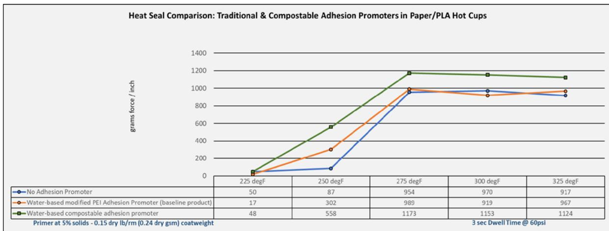
Figure 4: Heat-seal performance comparing traditional PEI adhesion promoter to CAP
