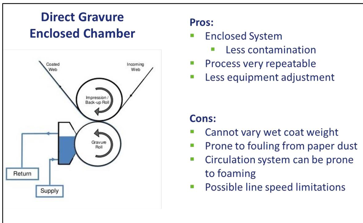
*Figure 7: Enclosed Chamber with Direct Gravure Applicator*
